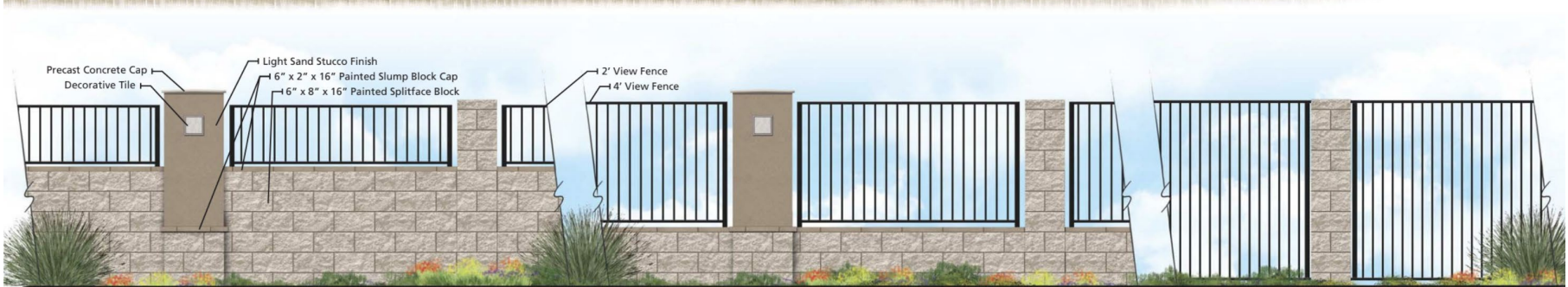
2' VIEW FENCE OVER 4' BLOCK WALL
